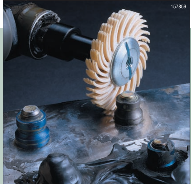
2" SR Radial Bristle Disc cleaning final layer of seam sealant around aircraft fuel tank fasteners.
