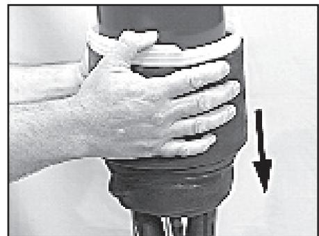
8.15 Continuously push PST tube downward while pulling the rest of the core material.
