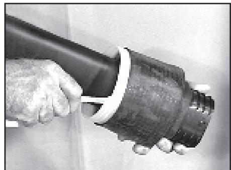
7.8 While holding the 3M™ Reenterable PST Dome Closure and closure with one hand, unwind the core by pulling on the core tail with the other hand in an upward and outward COUNTERCLOCKWISE direction until approximately 0.5"(13 mm) of the PST is shrunk onto the closure.
