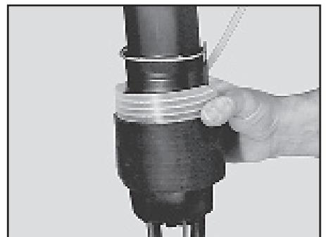
7.12 Continuously push PST tube downward while pulling the rest of the core material.
