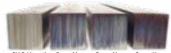
This photo shows four identical 304 stainless steel bars after nine grinding cycles of ten seconds each. While the three bars were ground using conventional ceramic abrasive belts show varying degrees of oxidation, the bar ground with a Cubitron II belt is free of burnishing.
