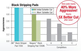
\*Pads worn via 50 passes over 3M™ Safety-Walk™ Slip-Resistant Treads 610 (swing machine)
