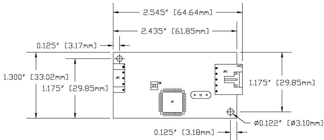
**Figure 4 EX151 Dimensions**
