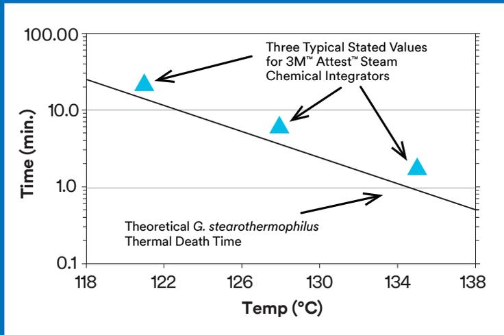
**Figure 1.** Graph comparing three typical Stated Values of 3M™ Attest™ Steam Chemical Integrators with the theoretical death curve of *Geobacillus stearothermophilus* spores.
