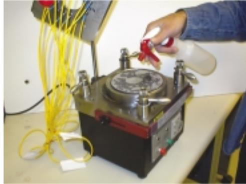
4. Wipe the surface of the 3M™ Lapping Film with a clean tissue. The goal here is to remove the air bubbles, smooth out the film and clean the surface of the film. The film should be wiped until almost completely dry and laying flat. This photo shows the film well adhered to the back-up pad, laying smooth and clean.
