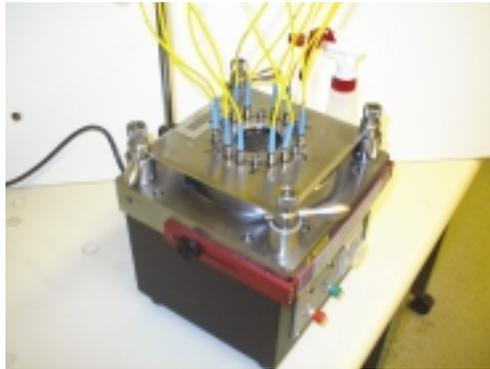
After the cycle, carefully lift the fixture, to minimize scoring of the film. The film can be wiped dry, and placed in an area for the next use.
