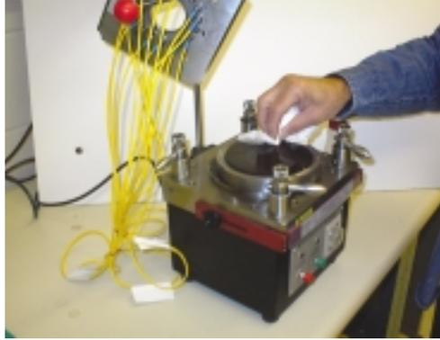
**Note:** The rubber back-up pad should be in good condition, with no scratches, gouges or foreign material on the surface. Additional cleaning or replacement may be necessary.
