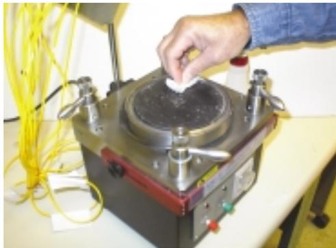
5. Blow the surface of the film completely dry with clean air or nitrogen to help remove any particulates that may have settled on the film. Apply de-ionized or distilled water. Using about 3 pumps of the spray bottle or enough to cover the surface of the film.
