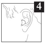
Here is the disposable ear plug properly positioned in the ear canal. For best fit, at least 1/2 to 3/4 of the ear plug should be inside your ear canal.
