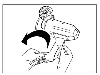
**6.** Hold the trigger and the air hose up into the upper housing and lift off – at the same time flipping it over so the interior is visible – and lay it next to the lower housing.
