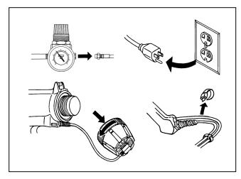
Disconnect air and electrical power and allow the applicator to cool to room temperature before disassembly.
