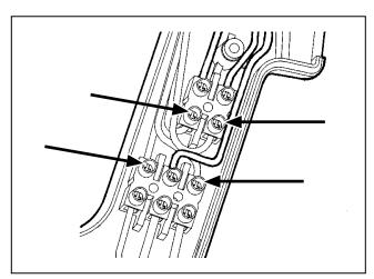
**8.** Loosen the three terminal block screws indicated by arrows about 3-4 turns. Either a 1/8 in. slotted blade screwdriver or a Phillips (P1) screwdriver can be used. Use a needle-nosed pliers and pull each wire out of the terminal blocks.
