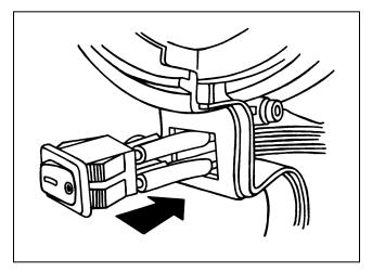
**11.** Feed the wire leads of the replacement switch through the opening of the housing. Position the switch so the leads with the red, silicone rubber sleeving are towards you.
