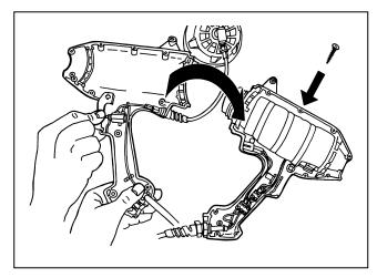
20. Hold trigger and the air hose in position in the upper housing and lift and turn the upper housing over onto the lower housing. Crossing the hands as shown will make it easier to hold the components in position while turning the housing over.
