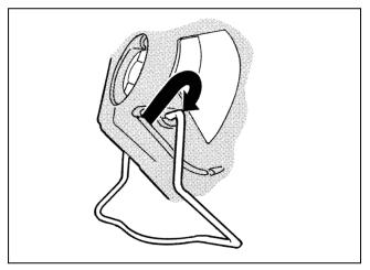
**25.** Pull the first end of the wirestand – from step 23 – out of the recess and position it over its pivot hole. The spring action of the wirestand will pull itself down into place.
