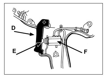
**18.** On the upper housing, make sure the trigger (D) is engaged on the valve button (E) and the trigger is positioned properly in its bearing.
