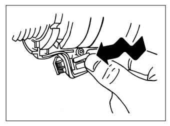
**10.** Grasp the switch and rock it back and forth while pushing it out of the hole in the housing
