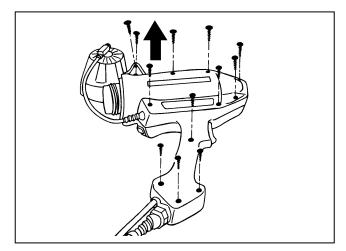
**4.** Remove the 12 screws that hold the housing halves together and save them for reassembly.
