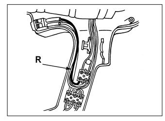
**16.** Bend the red wire (R) and route as shown. (The red wire is shown darker for clarity.)
