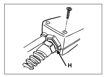
**21.** Separate the housing halves at the bottom of the handle just enough to adjust the position of the power cord strain relief. The hex (H) should be aligned and fully engaged with the matching hex-shaped recess in the housings. If necessary, rotate the strain relief hex one flat in either direction to obtain good fit.
