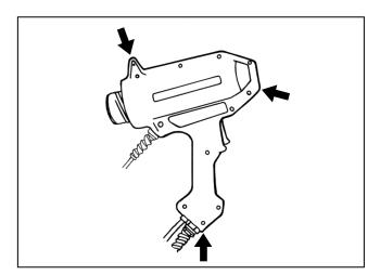
**5.** To make sure the upper housing will lift off cleanly, just **slightly** separate the two halves at the locations shown.
