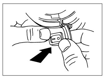
**12.** Push both sides of the switch bezel firmly until the switch snaps into place and is flush against the housing.
