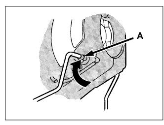
**24.** Pull the other end of the wirestand just enough to go over the edge of the applicator and position it into the pivot hole (A). The spring action of the wirestand will pull itself down into place.
