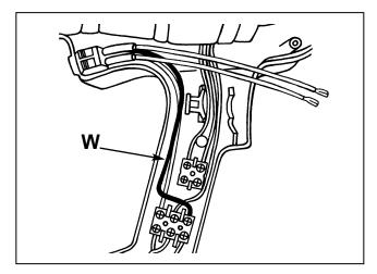
**14.** Bend the white wire (W) and route as shown. (The white wire is shown darker for clarity.)
