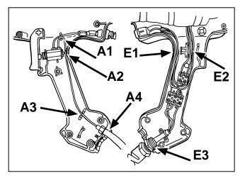
**19.** Check the locations indicated by arrows above to make sure all components are positioned properly.
