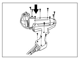
22. Recheck proper fit and alignment between the housing halves and make sure the trigger pivots freely.
