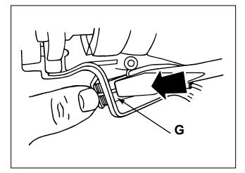
**9.** Press a large straight blade screwdriver - or other flat tool - down against both flexible retention springs (G). At the same time rotate the near side of the switch out of the opening in the housing.
