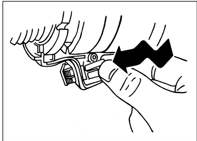
10. Grasp the switch and rock it back and forth while pushing it out of the hole in the housing
