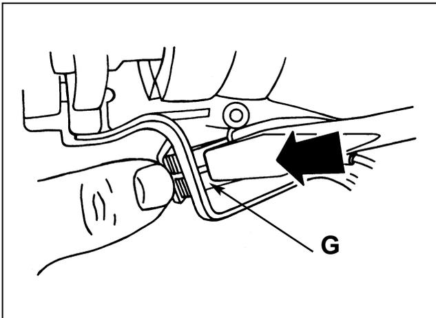
9. Press a large straight blade screwdriver - or other flat tool - down against both flexible retention springs (G). At the same time rotate the near side of the switch out of the opening in the housing.
