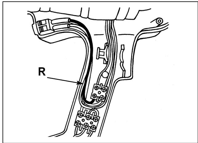
**16.** Bend the red wire (R) and route as shown. (The red wire is shown darker for clarity.)
