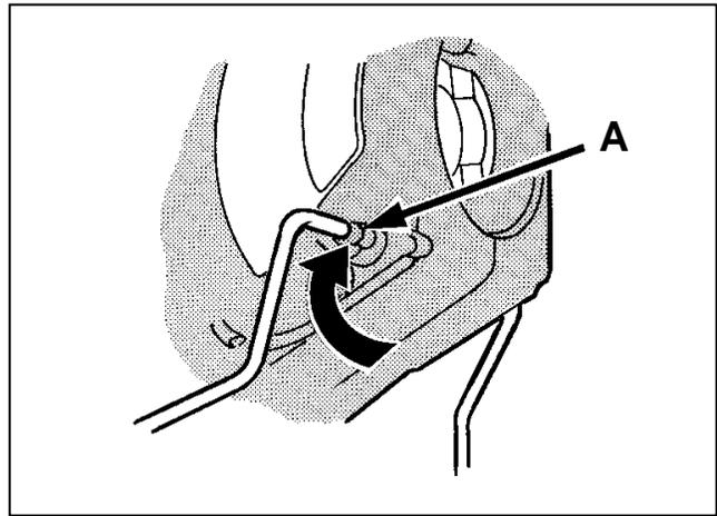
**24.** Pull the other end of the wirestand just enough to go over the edge of the applicator and position it into the pivot hole (A). The spring action of the wirestand will pull itself down into place.
