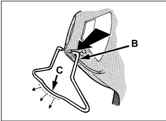
**23.** Hold the wirestand so the rounded part (C) curves away from the applicator and temporarily hook one end of the wirestand so the end rests down in the bottom of the recess (B) as shown.
