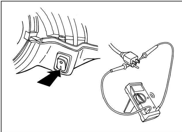
**17.** Check for proper electrical installation by connecting a multimeter or continuity tester across the power cord plug blades. Continuity should exist when the switch is pushed to the on position.
