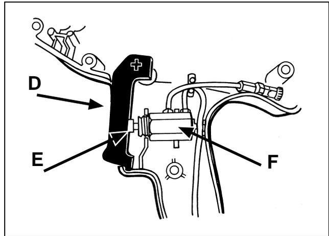
**18.** On the upper housing, make sure the trigger (D) is engaged on the valve button (E) and the trigger is positioned properly in its bearing.
