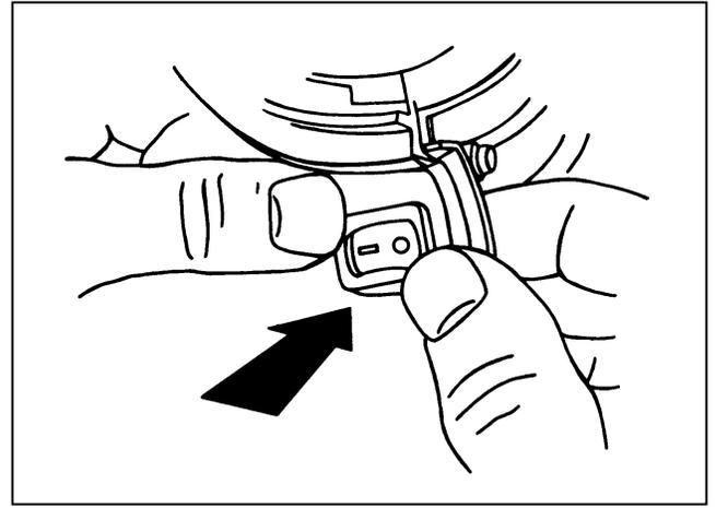
**12.** Push both sides of the switch bezel firmly until the switch snaps into place and is flush against the housing.
