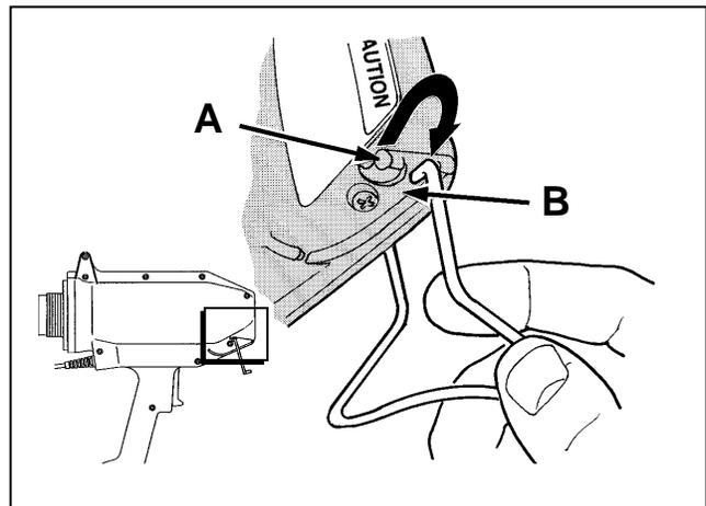
2. Pull one side of the wirestand out of the pivot hole (A) and allow it to spring down into the recessed area (B).
