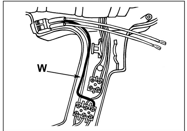
**14.** Bend the white wire (W) and route as shown. (The white wire is shown darker for clarity.) Twist the end connector (A) on the wire so the wide sides are horizontal as shown in step 13. Insert the wire about 1/4 in. (6.4 mm) into the hole on the right side of the 3-pole terminal block and tighten the screw firmly.
