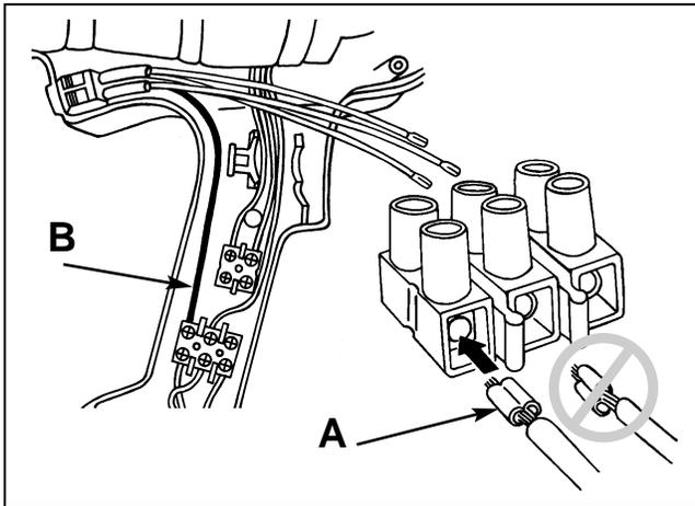
**13.** Route the black switch wire (B) as shown. Twist the end connector (A) on the wire so the wide sides are horizontal. Insert the wire about 1/4 in. (6.4 mm) into the hole on the left side of the of the 3-pole terminal block and tighten the screw firmly.
