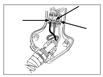
**8.** Loosen the three terminal block screws indicated by arrows about 3-4 turns. Either a 1/8 in. slotted blade screwdriver or a Phillips (P1) screwdriver can be used.
