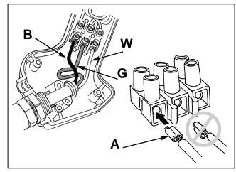
**10.** Twist the end connectors (A) of the replacement power cord so the wide sides are horizontal.
