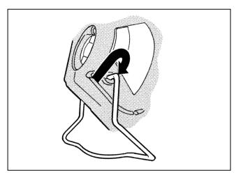
**20.** Pull the first end of the wirestand – from step 18 – out of the recess and position it over its pivot hole. The spring action of the wirestand will pull itself down into place.
