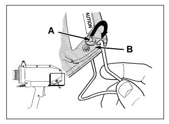
**2.** Pull one side of the wirestand out of the pivot hole (A) and allow it to spring down into the recessed area (B).
