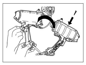
**15.** Hold trigger and the air hose in position in the upper housing and lift and turn the upper housing over onto the lower housing. Crossing the hands as shown will make it easier to hold the components in position while turning the housing over.
