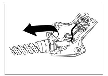
**9.** Pull the faulty power cord up slightly to allow the strain relief to clear the recesses in the housing and then straight back to remove completely.
