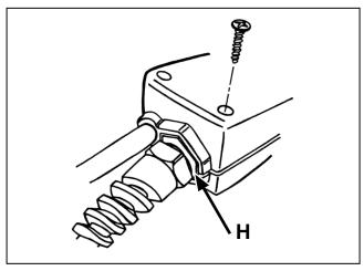
**16.** Separate the housing halves at the bottom of the handle just enough to adjust the position of the power cord strain relief. The hex (H) should be aligned and fully engaged with the matching hex-shaped recess in the housings. If necessary, rotate the strain relief hex one flat in either direction to obtain good fit.
