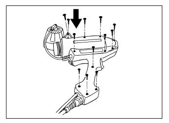
**17.** Recheck proper fit and alignment between the housing halves and make sure the trigger pivots freely.
