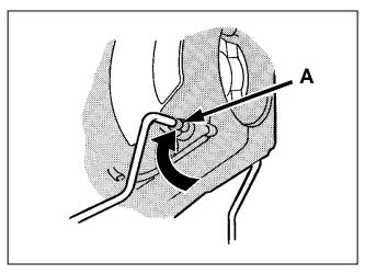
**19.** Pull the other end of the wirestand just enough to go over the edge of the applicator and position it into the pivot hole (A). The spring action of the wirestand will pull itself down into place.
