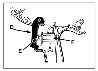
**12.** On the upper housing, make sure the trigger (D) is engaged on the valve button (E) and the trigger is positioned properly in its bearing.
