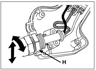
**14.** The proper position of the power cord end and the strain relief is shown above. The hex (H) is fully engaged in the matching hex-shaped recess in the housing. If necessary, lift the strain relief up and rotate it one flat in either direction to obtain a good fit.
