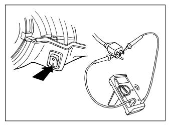
**11.** Check for proper electrical installation by connecting a multimeter or continuity tester across the power cord plug blades. Continuity should exist when the switch is pushed to the on position.
