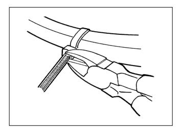
21. The plastic tie wraps provided can be used to hold the power cord and the air supply hose together.
