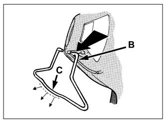
**18.** Hold the wirestand so the rounded part (C) curves away from the applicator and temporarily hook one end of the wirestand so the end rests down in the bottom of the recess (B) as shown.
