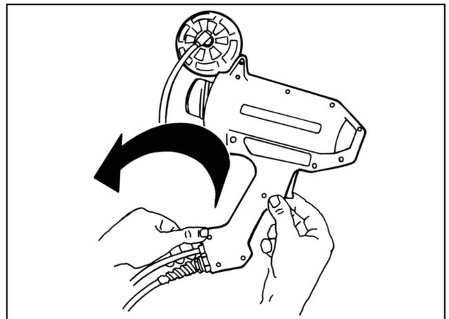
6. Hold the trigger and the air hose up into the upper housing and lift off – at the same time flipping it over so the interior is visible – and lay it next to the lower housing.
