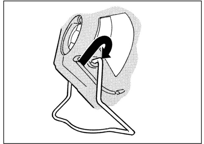
**20.** Pull the first end of the wirestand – from step 18 – out of the recess and position it over its pivot hole. The spring action of the wirestand will pull itself down into place.
