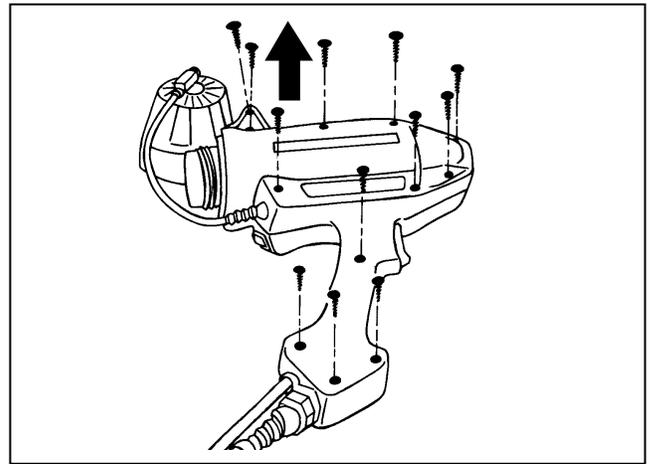
4. Remove the 12 screws that hold the housing halves together and save them for reassembly.
