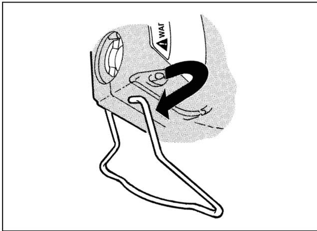
3. Turn the applicator over and pull the other side of the wirestand out of the other pivot hole and over the edge of the applicator.
