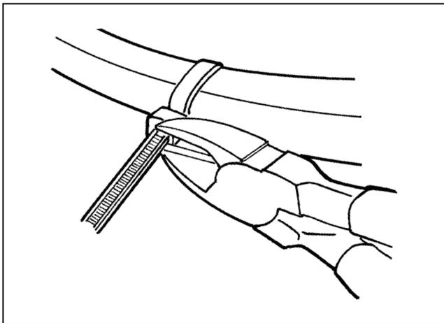
**21.** The plastic tie wraps provided can be used to hold the power cord and the air supply hose together. With the smooth side facing out, attach the first tie wrap about 6 in. (15 cm) from the applicator and space the others about 24 in. (61 cm) apart. Make sure you trim the tails of the tie wraps carefully so there are no sharp edges.
