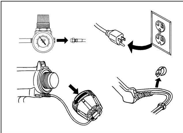
1. Disconnect air and electrical power and allow the applicator to cool to room temperature before disassembly.
