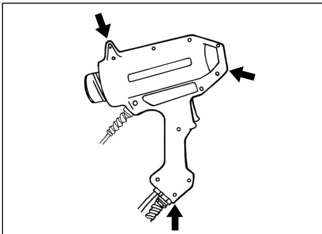
5. To make sure the upper housing will lift off cleanly, just **slightly** separate the two halves at the location shown.
