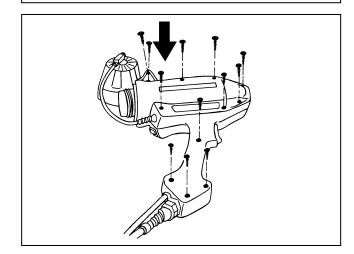
**23.** Recheck proper fit and alignment between the housing halves and make sure the trigger pivots freely.
