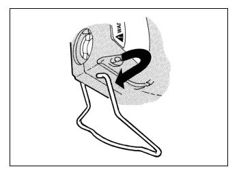
**3.** Turn the applicator over and pull the other side of the wirestand out of the other pivot hole and over the edge of the applicator.
