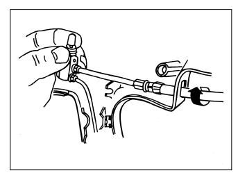
**15.** Insert the tubing end of the endcap air hose through the opening in the housing.
