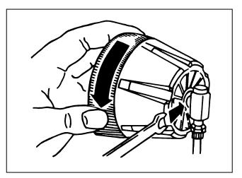
**27.** Reattach endcap to quick dump valve by holding fitting with wrench and turning endcap in direction shown.
