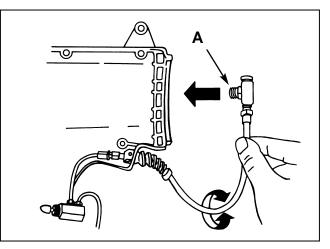
**17.** Twist the endcap hose so the quick dump valve will lie flat on the work surface and fitting (A) will be directed straight down the center of the housing when the hose is bent up into the position shown above.
