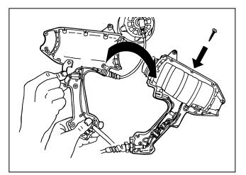
**21.** Hold trigger and the air hose in position in the upper housing and lift and turn the upper housing over onto the lower housing. Crossing the hands as shown will make it easier to hold the components in position while turning the housing over.
