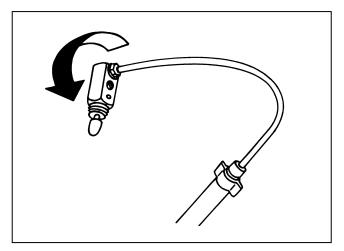
**13.** Attach the **replacement air valve** to the air supply tubing by screwing the valve on the fitting.
