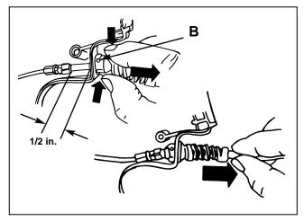
**16.** Position the strain relief so that it is about 1/2 in (12.7 mm) from the hose fitting as shown.
