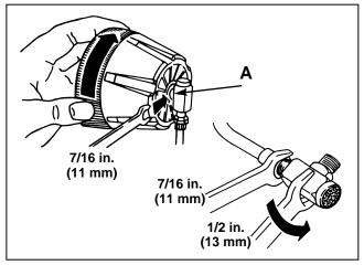
**8.** Unscrew the endcap from the quick dump valve by holding fitting (A) and turning in the direction as shown.
