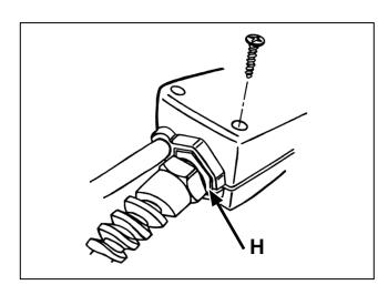
**22.** Separate the housing halves at the bottom of the handle just enough to adjust the position of the power cord strain relief. The hex (H) should be aligned and fully engaged with the matching hex-shaped recess in the housings. If necessary, rotate the strain relief hex one flat in either direction to obtain good fit.
