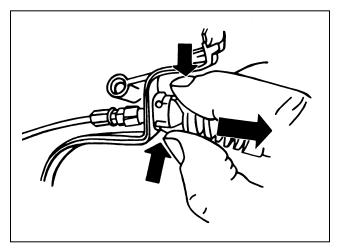
**12.** Squeeze the upper and lower parts of the strain relief together and at the same time, pull it out of the housing. Discard the hose and all connected fittings and strain
