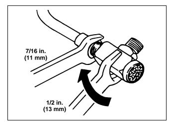
**14.** Attach the quick dump valve from step 8 to the replacement air hose.
