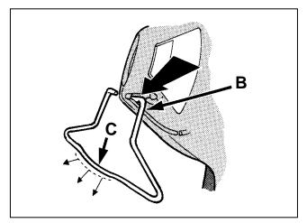
**24.** Hold the wirestand so the rounded part (C) curves away from the applicator and temporarily hook one end of the wirestand so the end rests down in the bottom of the recess (B) as shown.
