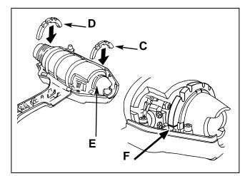
7. If the front standoff (C) or the rear standoff (D) is dislodged in any way, replace them on the heat tube (E). Upper and lower sets of standoffs should be in contact with no visible gaps between them at all four locations (F).
