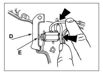
**19.** Place the valve in position and press the tubing down into the grooved ribs as shown. The tubing on the replacement air supply line should be underneath the tubing that connects to the endcap.
