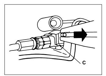
**11.** Pull the tapered locking pin out of the air hose strain relief (C).
