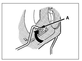
**25.** Pull the other end of the wirestand just enough to go over the edge of the applicator and position it into the pivot hole (A). The spring action of the wirestand will pull itself down into place.
