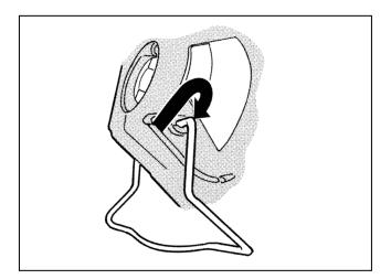
**26.** Pull the first end of the wirestand – from step 24 – out of the recess and position it over its pivot hole. The spring action of the wirestand will pull itself down into place.
