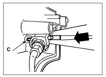
**18.** Push the smaller diameter end of the tapered locking pin into the hole in the strain relief.
