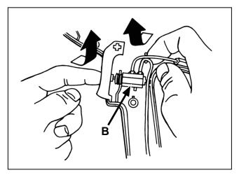
**9.** Pull the valve (B) out of the upper housing by lifting the tubing out of the notched ribs and lifting up on the trigger.
