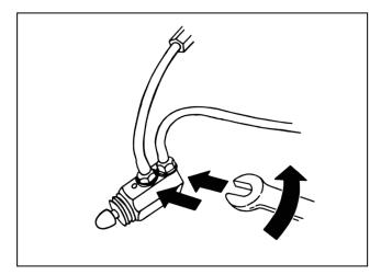
**10.** Use a 1/4 in. open end wrench and remove the brass fitting that connects the air supply tubing to the valve.
