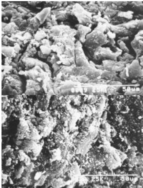
Figs. 10 and 11: SEM picture of a sand-blasted resin surface (Bioplus-Zahn, Detrey) after microblasting (Rocatec Pre, 110 \mu\text{m} ) [Fig. 10] and after coating (Rocatec Plus) [Fig. 11], magnified 1000x.
