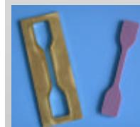
Specimen acc. to DIN 53504
