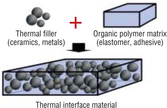
Most thermal interface materials—including thermal pads, tapes, phase change materials and epoxies—consist of ceramic or metal particles suspended in an organic polymer. Thermal conductivity increases with filler density.
