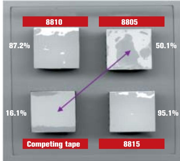
3M's Series 8800 thermally conductive adhesive transfer tapes have excellent wetting ability. In this test, the tapes were used to bond an aluminum heat sink to a glass slide. All three tapes adhered to significantly more of the slide than a competing tape.
