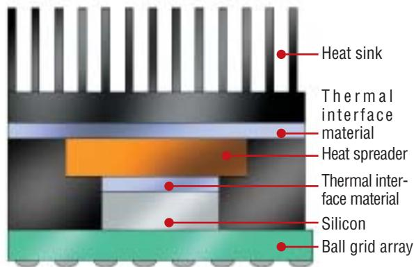
**The silicon chip inside a ball grid array can generate enough heat to degrade its functionality. Heat spreaders and heat sinks dissipate this heat. To ensure efficient heat transfer, a thermally conductive material must be inserted between the silicon and the heat spreader, and between the heat spreader and the heat sink. This material can be an adhesive or some other thermally conductive material.**
