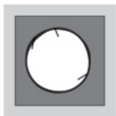
D1 hole with burr from mechanical punch
