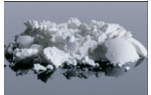
Conventional glass ionomer powder becomes compacted during storage and when dispensed with the spoon; dosing is not consistent.
