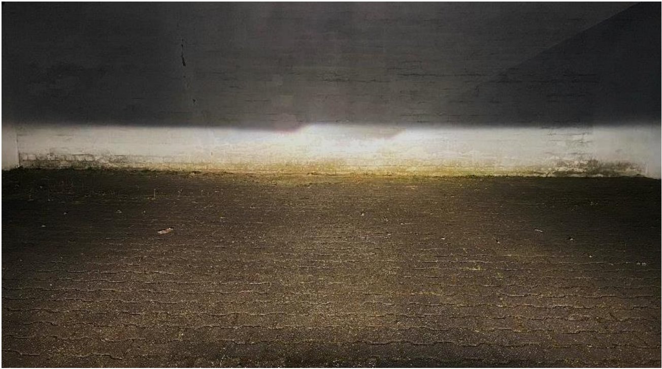
Figure 5: Typical ECE passing beam light distribution with pronounced cut-off line for typical sign locations / HID Projector Lens / Model Year 2015 [11].
