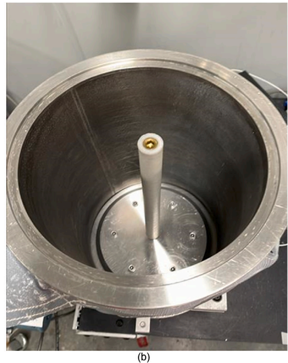
Fig. 1. Experimental Set Up. (a) Schematic illustrating the gas evacuation path and position of a single pressure gauge; and (b) Photograph of stainless-steel cylinder interior where the filter (sintered HDPE porous tube) can be seen.
