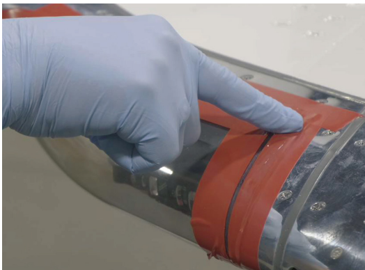
Figure 14: Edge seal can be smoothed after application.
