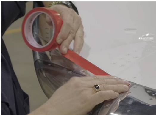
Figure 12: Apply masking tape to enable neat edge seal application.
