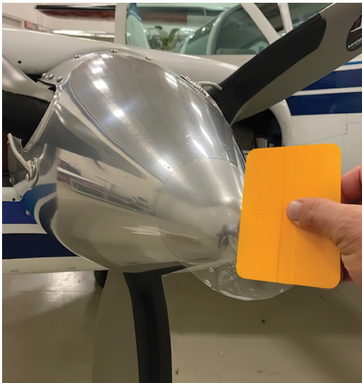
Figure 11: Representative image — Applying and smoothing out boot with the yellow squeegee.
