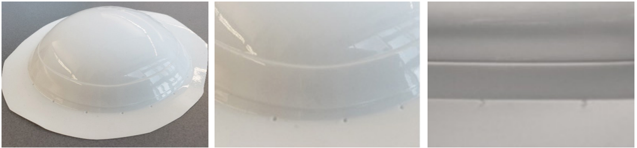
Figure 1: Representative trim lines provided on boots.
