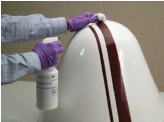
Figure 3: Representative image — Cleaning dome and boot.
