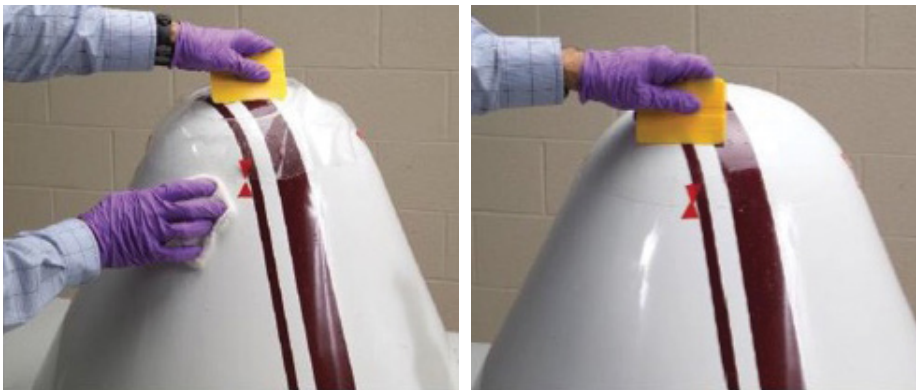
Figure 10: Representative image — Process of smoothing out boot with the yellow squeegee.
