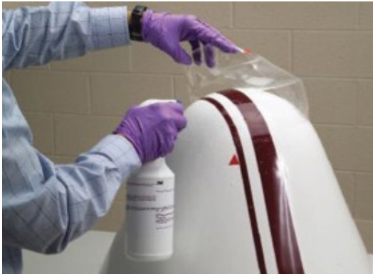
Figure 8: Representative image — Spraying dome surface with 3M™ Protective Tape Application Solution.
