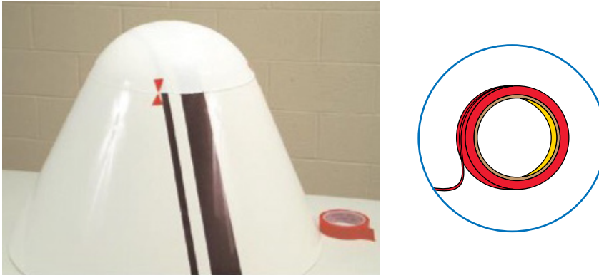
Figure 6: Representative image — Placement of alignment marks on dome and boot.
