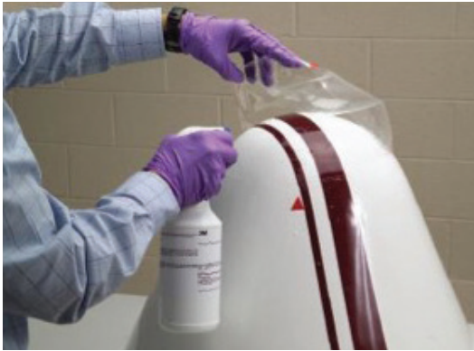
Figure 8: Representative image - Spraying radome surface with 3M™ Protective Tape Application Solution.
