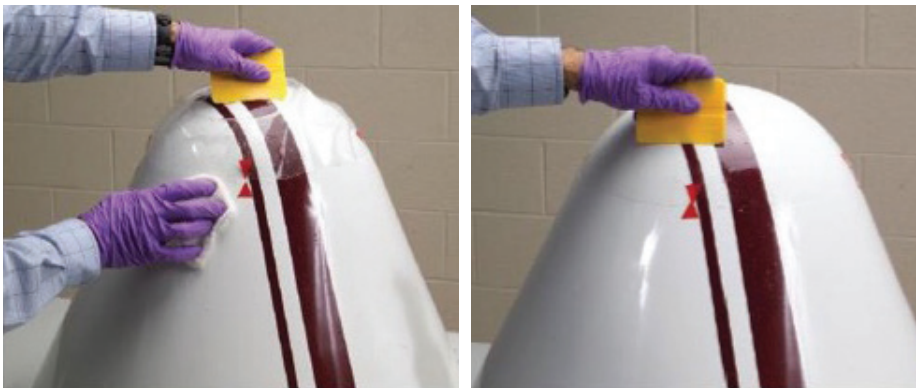
Figure 10: Representative image - Process of smoothing out boot with the provided squeegee.
