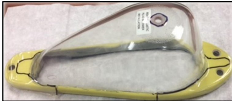
Figure 1 In Process Installation of Light Lens Boot
