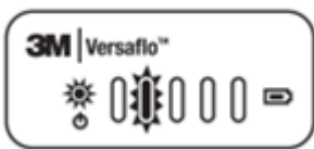
Figure 3: Poor electrical contact
