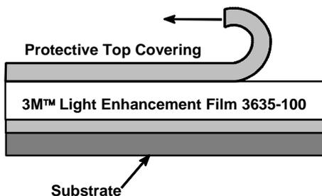
**Figure 2. Removing Protective Top Covering from 3M™ Light Enhancement Film 3635-100**
