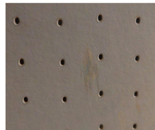
Impact on area protected by 3M Tape 8642 without perforation. Image courtesy of Sergent-Chef Marzin Loic, ©L.Marzin/Armée de l'Air. Reproduced with permission.
