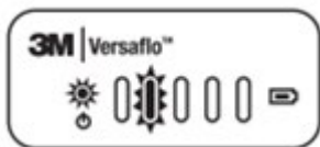
Figure 3: Poor electrical contact
