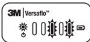
Figure 4: No electrical contact
