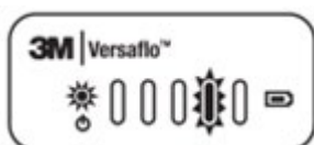
Figure 1: Battery outside of temperature range
