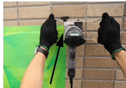
Figure 14. Align the notch in the TSA-4 tool with the bottom of the previous pass to ensure a 50% pass overlap
