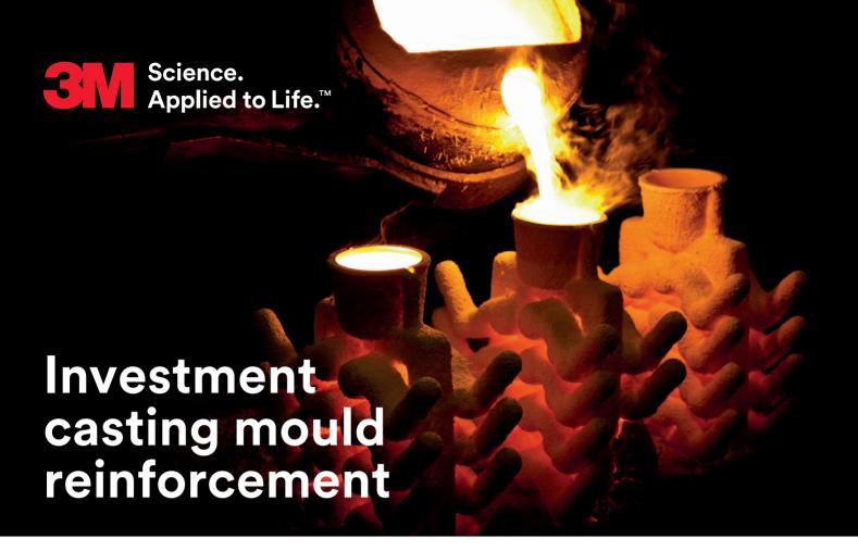
3M™ Nextel™ Ceramic Textiles can be used to reinforce moulds to help prevent failures in casting and control cooling.
