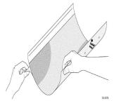
Figure 8. Lift the graphic and peel back the liner.
