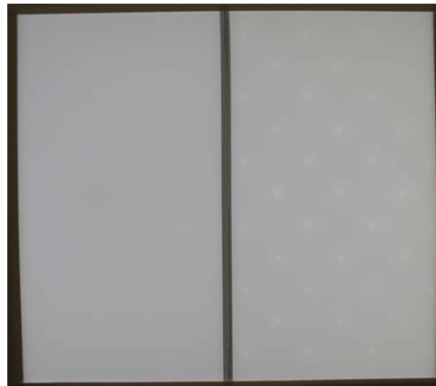
Figure 4. LED Hiding Capabilities of Diffuser Films
