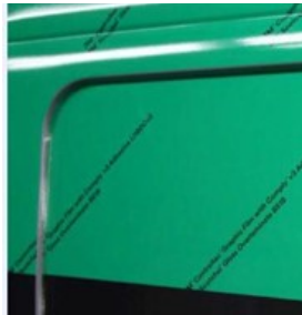
Figure 24. Finished Relief Cut
