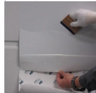
Figure 15. Unrolling the Liner While Applying Film
