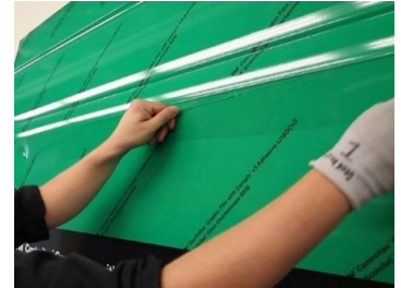
Figure 22. Cutting With 3M™ Knifeless™ Tape
