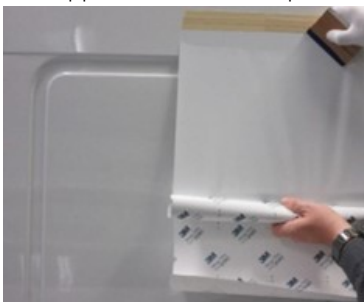
Figure 13. Aligning and Attaching the Panel with Masking Tape
