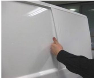
Figure 9. Aligning Contour Edges
