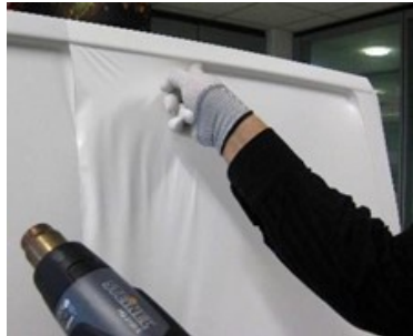
Figure 11. Applying Heated Film to the Recess
