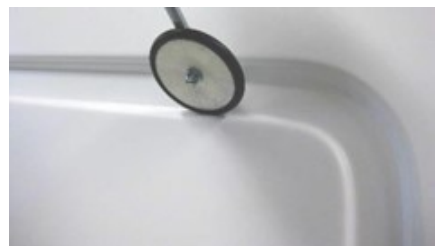
Figure 20. Re-rolling Recessed Film
