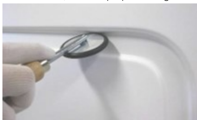
Figure 20. Re-rolling Recessed Film
