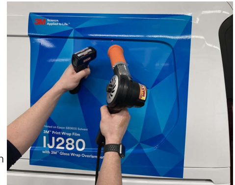
Figure 2. Heating the Film and Measuring the Temperature
