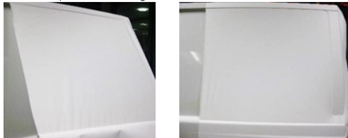
Figure 8. Positioning and Tacking the Film to a Single Recess
