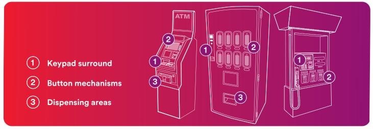
3M™ Industrial Protective Film 7070UV can be used in common wear areas to help protect the surfaces from moisture, scratches and UV rays.
