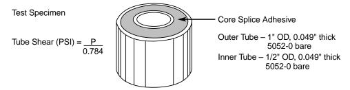
**Cure Cycle A:**  $250^{\circ}F$  ( $121^{\circ}C$ ) - 0 psig - 120 min.  $- 7.5^{\circ}F$ /min. warmup. **Cure Cycle B:**  $350^{\circ}F$  ( $177^{\circ}C$ ) - 0 psig - 60 min.  $- 7.5^{\circ}F$ /min. warmup.
