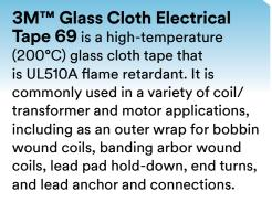
Designed for continuous operation not exceeding 200°C (392°F) per UL listing and 180°C (356°F) per CSA listing.
