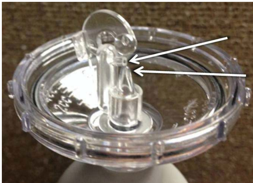
Figure B. Locations of two narrow passageways that must be cleaned with small-gauge wire.
