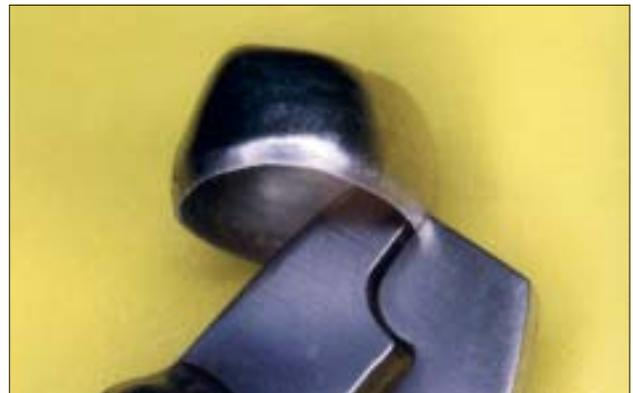
Figure 6. The crimping pliers bends edges inwardly.
