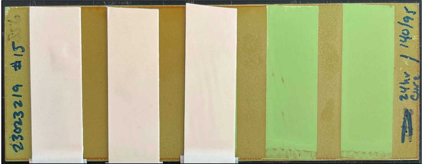
Figure 48 Representative image of CIC-coated panel after removal of 9143FR after exposure “Hot/Wet” dwell conditions (aegr021523-064)
