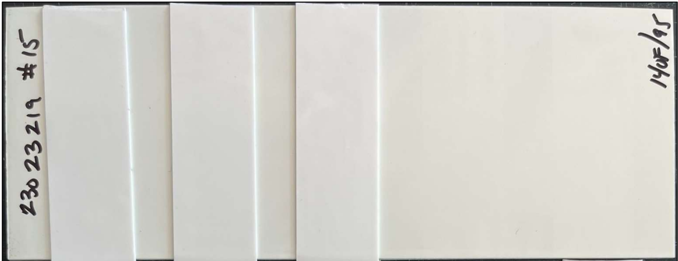
Figure 38 Representative image of epoxy topcoat panel after removal of 9143FR after exposure to “Hot/Wet” dwell condition (aegr021523-058)
