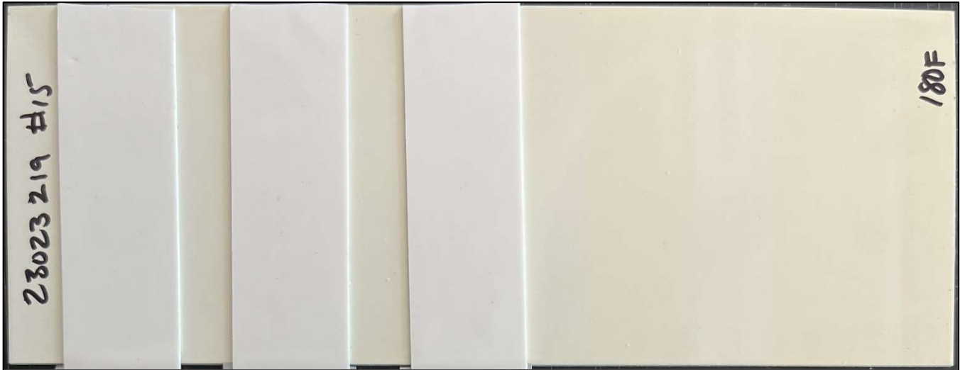
Figure 37 Representative image of epoxy topcoat panel after removal of 9143FR after exposure to “Dry Heat” dwell condition (aegr021523-057)
