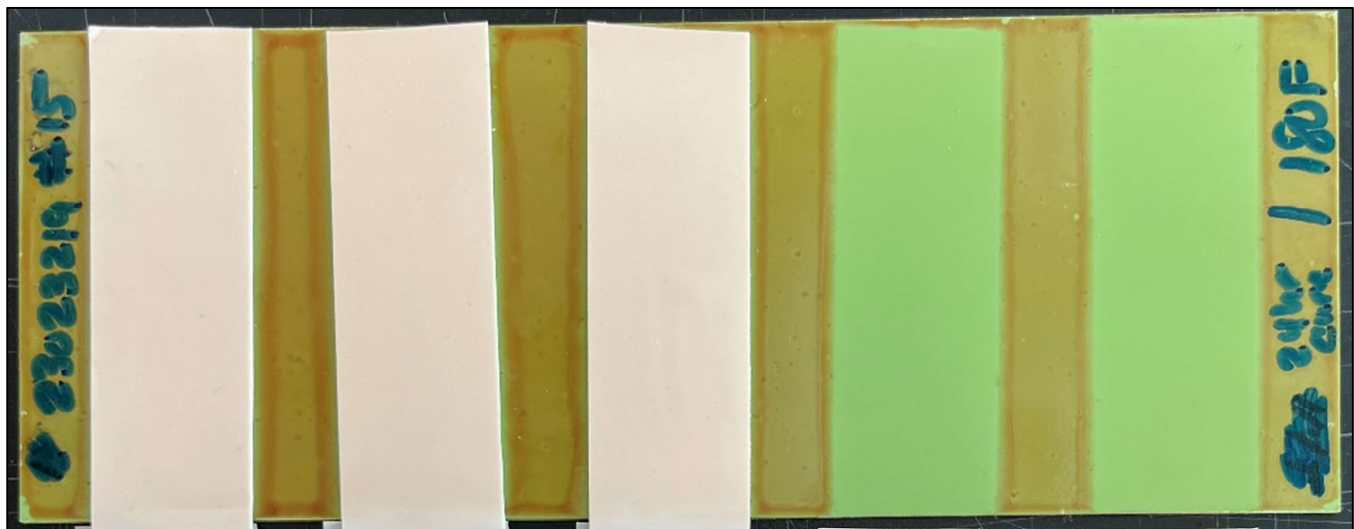
Figure 47 Representative image of CIC-coated panel after removal of 9143FR after exposure "Dry Heat" dwell conditions (aegr021523-063)
