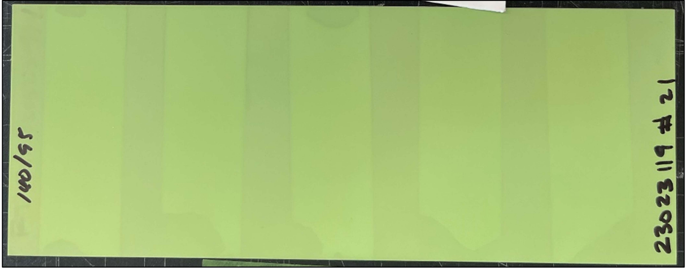
Figure 36 Representative image of epoxy-primed panel after removal of 9143FR after exposure to “Hot/Wet” dwell condition (rema020723-014)
