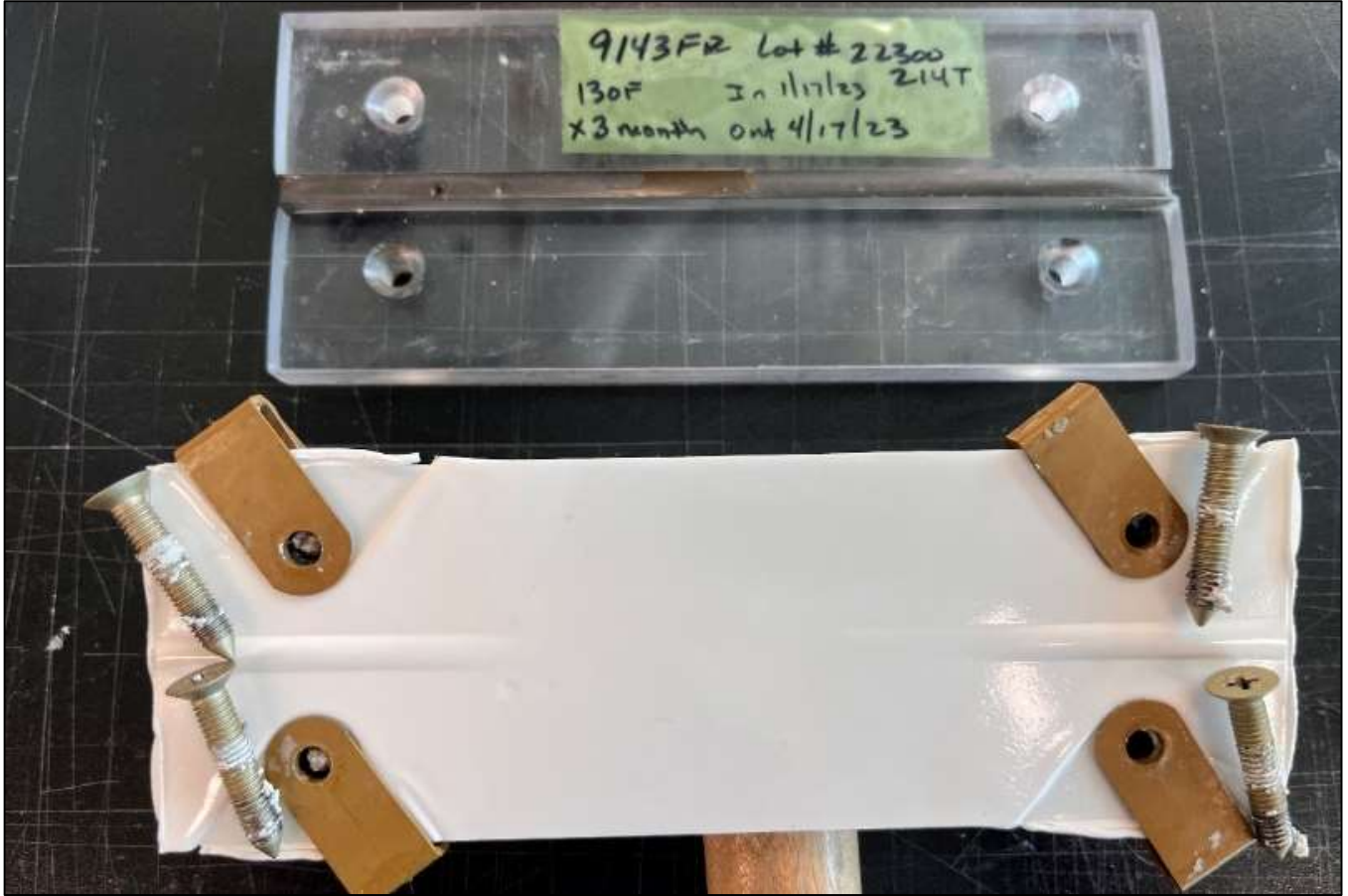
Figure 44 Simulated Floor Construction After Aging with Acrylic Panel Removed
