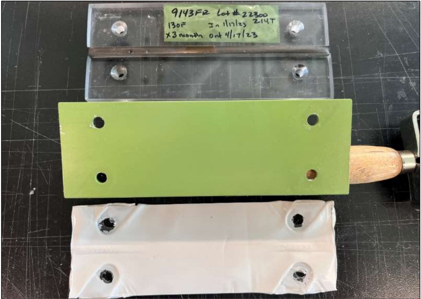
Figure 45 Simulated Floor Construction with 9143FR removed after 3 months aging at 130 °F
