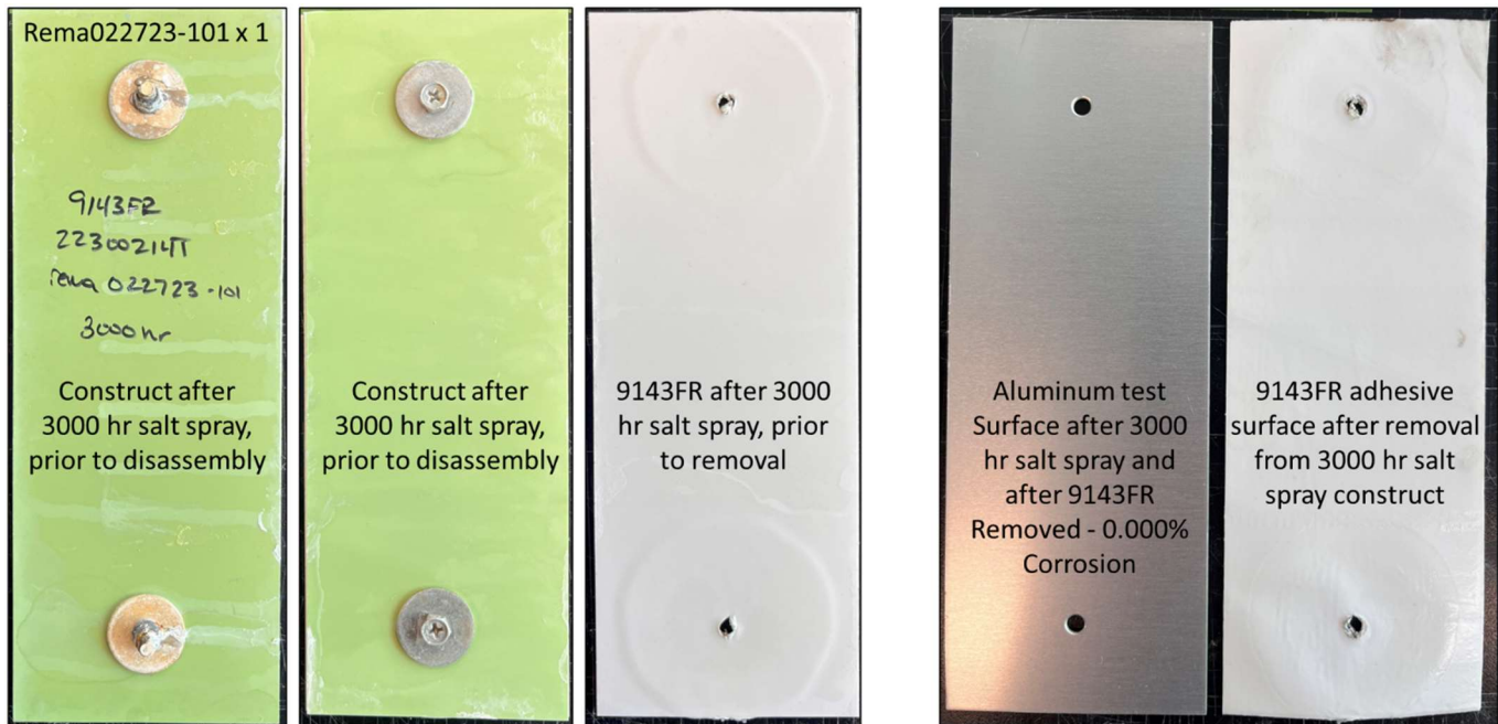
Figure 9 Example images of each step of corrosion construction disassembly after 3000 hours salt spray
