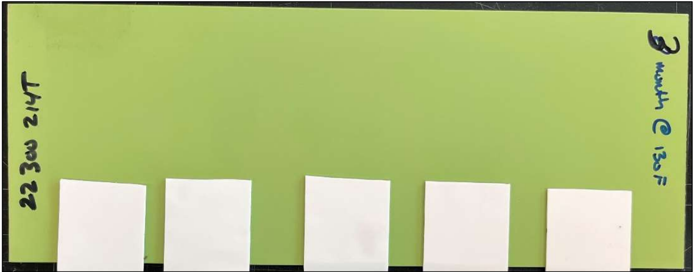
Figure 39 Representative image of epoxy-primed panel after removal of 9143FR after exposure to 130 °F for 3 months (aegr011723-908)
