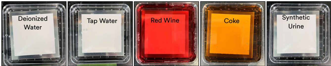
Figure 3 Images of submerged fluid soak sample prior to exposure
