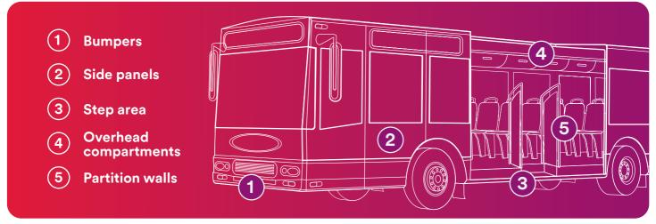
3M™ Industrial Protective Film 7070UV can be used in common wear areas to help protect the surfaces from moisture, dirt and UV rays.
