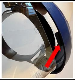
The arrow points to the latch feature. If you have affected product, this is the location that the faceshield would not attach to the headgear properly.
