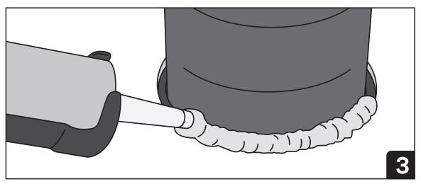
Seal the system with 3M<sup>™</sup> Fire Barrier Sealant applied to appropriate interfaces as per system specifications.
