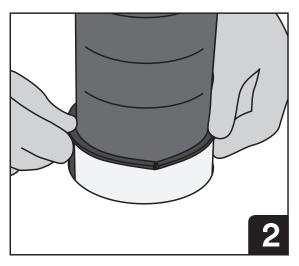
Wrap Tuck-In around pipe and position according to system requirements. Secure with provided adhesive installation tab or equivalent.
