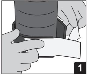
Measure and cut Tuck-In Wrap Strip to appropriate length (or use pre-cut wrap strips) for pipe size and layers required as per system specifications.
