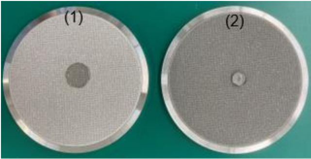
Fig. 1 Coating effectiveness at water protection on pad conditioners (1) Uncoated 3M diamond pad conditioner (2) 3M diamond pad conditioner with a hydrophobic coating
