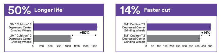
1. Results are based on an automated beveling of 1018 carbon steel bars. Grinding wheel geometry is 115mm outer diameter mounted on a servo motor with an applied force of 12 lbs. Cut speed is defined by metal removed after 10 minutes of testing. The total material removal is estimated based on the amount of wheel used for 10 minutes of testing life. End of life is assumed to be 50% of the initial wheel mass.
