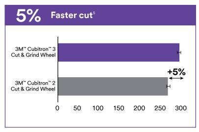
5. Results are based on an automated beveling of 1018 carbon steel bars. Cutting & grinding wheel geometry was 115mm outer diameter mounted on a servo motor with an applied force of 12 lbs. Cut speed is defined by metal removed after 10 minutes of testing. The total material removal is estimated based on the amount of wheel used for 10 minutes of testing life. End of life is assumed to be 50% of the initial wheel mass.
