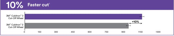
1. Results are based on an automated cutting of a 3mm thick 304 stainless steel sheet.
