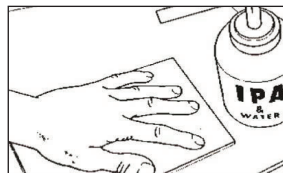
Step B: Solvent Wipe Note: Be sure to carefully read and follow solvent manufacturer's directions for use and precautions.
