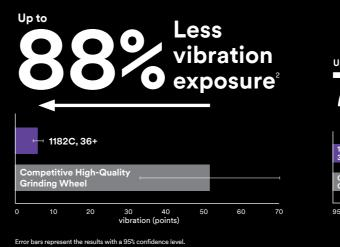
tive Shaped Grain Fibre Disc. Results are based on an automated, 30-minute, high pressure test on 1018 steel using 7 inch, 36+ grit fibre discs and Plate Ribbed 80514 on a servo
