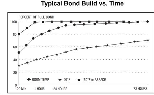
\*Note: Chart describes general performance of 3M<sup>™</sup> VHB<sup>™</sup> Tapes. Actual bond strength vs. time will depend on several factors including tape and substrate
