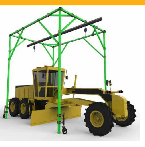
The Box Frame System is a mobile solution designed to be positioned manually. The freestanding design straddles the work surface, allowing the fall protection rails to run parallel with the work surface. This system will provide fall protection coverage over a large footprint or area. Available in adjustable height and fixed height models, this two-user solution can be utilized for a wide variety of applications.
