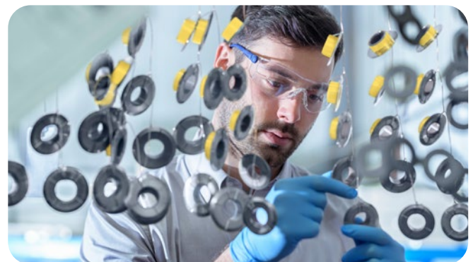
3M™ Vinyl Tape 471, shown here in yellow, can be used to mask part areas prior to a chemical bath, then removed cleanly upon process completion.
